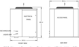
OC Refrigerant Connections: Discharge Line- 1/2", Liquid Line- 3/8"
